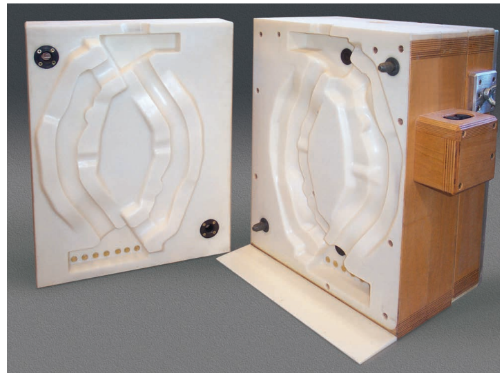
Core box made of SikaBiresin® UR132
