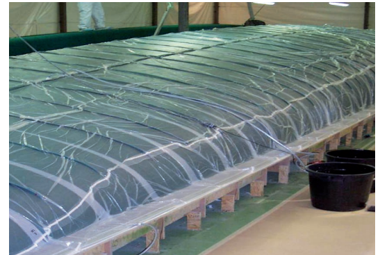
Vacuuminfusion with SikaBiresin® CR131
