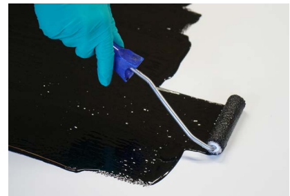
Roller application of SikaBiresin GC155
